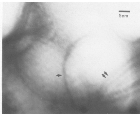
Figure 7 Micrograph of a microcrystalline calcium silicate hydrate, with a CaO/SiO 2 molar ratio of 1.65.
